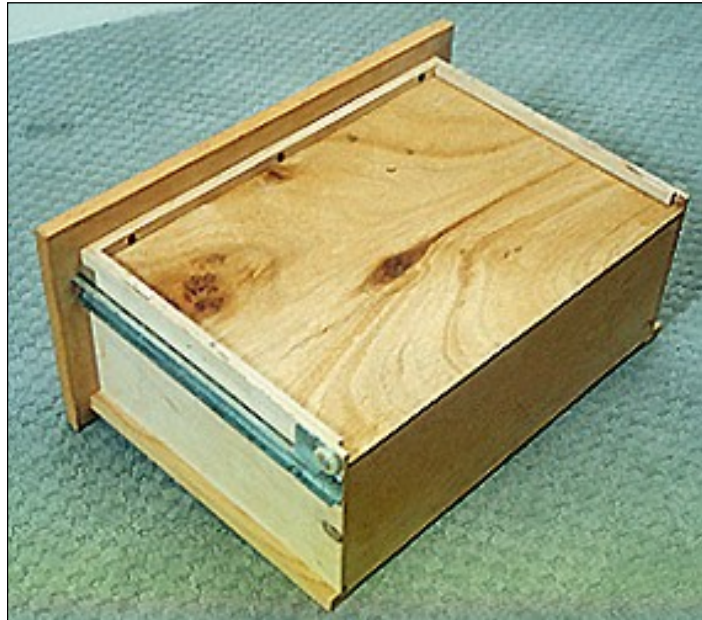
Figure 2. View of underside of drawer showing slides and 6 mm (1/4") plywood bottom held in grooves worked in drawer sides and front.
