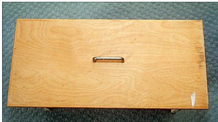
Figure 3. Front view of planted drawer front. Note plywood is lipped with an edging to hide veneer core.
