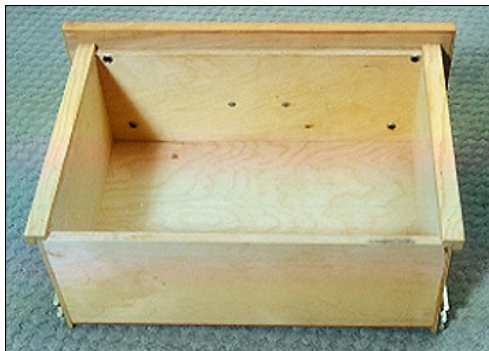
Figure 1. Simple plywood drawer with screwed on planted plywood front.
