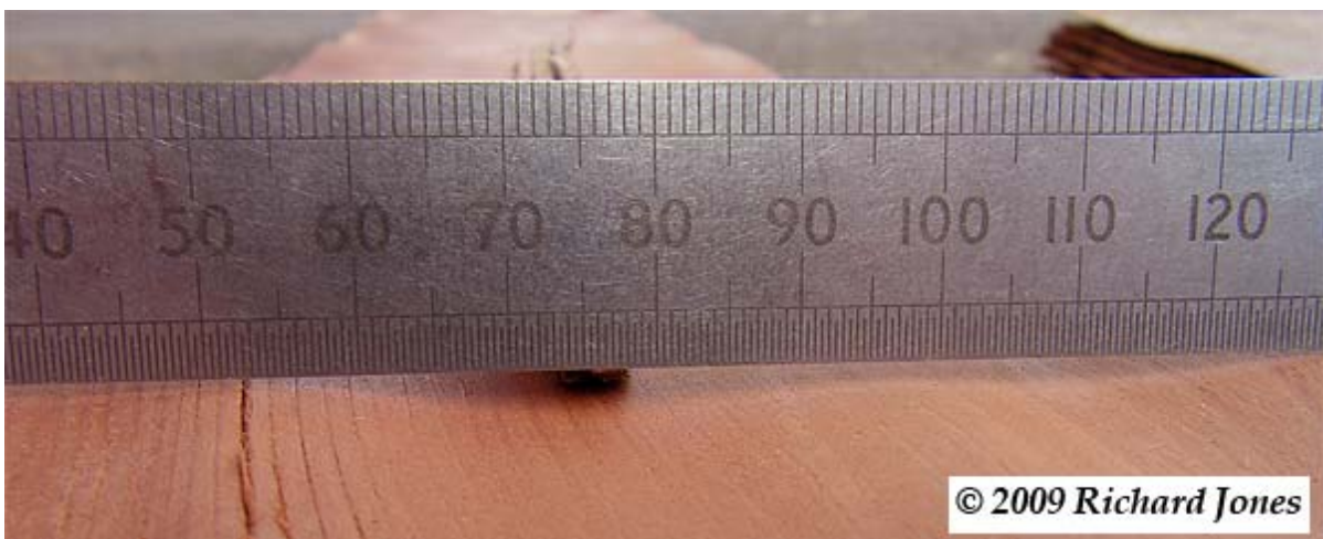
Below. A single gently cupped gap shows below the rule but this piece of yew veneer will lay flat without problems.
